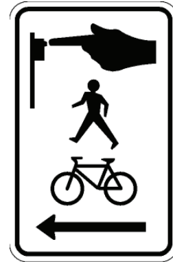
Figure 5.43 – Signalized Intersection Crossing Sign
