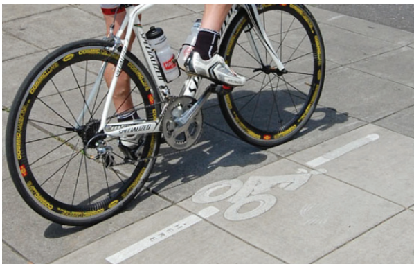
Figure 5.44 - Example Pavement Marking for Bicycle Actuation Location
